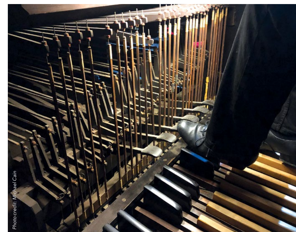
The foot pedals of the Erben organ, connected via a series of linkages to the long bass pipes.
